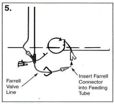
Insert FARRELL line connector into feeding tube.
